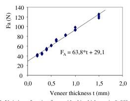
**Fig. 4** Variation of cutting force with chip thickness in 0–90° cutting mode (from Beauchêne 1996); the width of the chip is 20 mm. Force intercept with zero thickness is linked to specific work of surface separation which is dissipated whatever the very low thickness of chip
