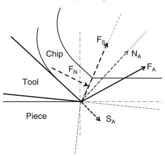
**Fig. 3** Force exerted by the tool on the chip  $(F_A)$ .  $N_A$  is the normal (compressive) rake force,  $S_A$  is the parallel (shearing) rake force,  $F_N$  is the normal (compressive) force to the shearing plane,  $F_S$  is the parallel (shearing) force to the shearing plane
