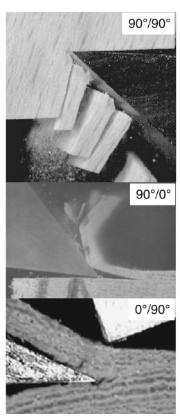
**Fig. 7** Discontinuous cutting with crack opening. **a** top: 90–90° cutting mode (Photo Pfeiffer R). **b** middle: 90–0° cutting mode (Photo Chardin A). **c** bottom: 0–90° cutting mode (Photo Thibaut B)
