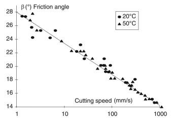
**Fig. 8** Evolution of friction angle with cutting speed for green wood (chestnut) at 2 temperatures (from Thibaut 1988). It should be noted that the *bottom left* of the graph is not a true origin (neither the ordinate nor the abscissa is zero), but the axes are shown intersecting by commodity; abscissa (cutting speed) is used in logarithmic scale, but the actual values are put in legend
