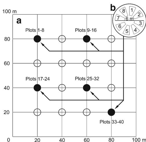
**Fig. 1** **a** Plot design to sample forest floor (dark circles—randomly chosen five intersections of grid where we established groups of eight soil plots; 40 in total). **b** Design of single soil plots group
